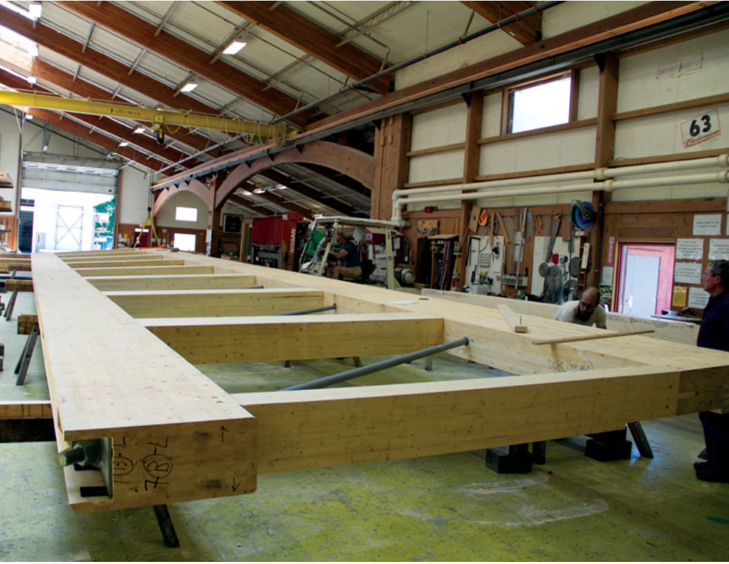
Mass timber structural element being produced. Photo courtesy of Alan Organschi.
