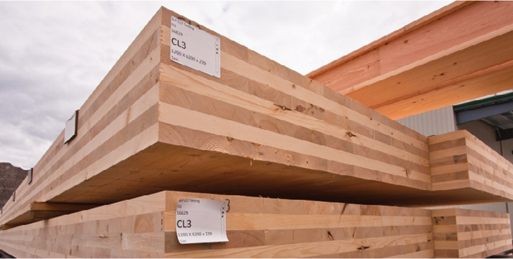
Cross-laminated timber is made from boards that have been glued together at opposing angles to increase strength. Photo courtesy of Steve Marshall.
