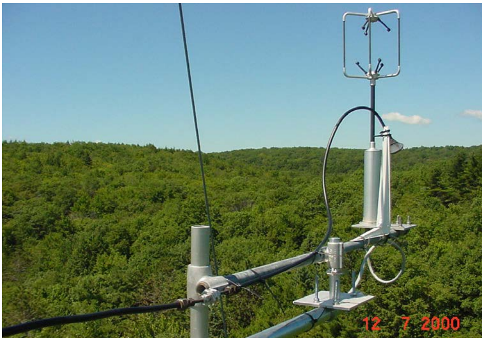
View of the sonic anemometers high above Great Mountain Forest. These devices detect pulses of ultrasonic sound waves as a means of measuring wind velocity. Other essential equipment includes the infrared gas analyzer for measuring the elements or molecules of interest, and a hygrometer for determining the relative humidity of wind samples.
