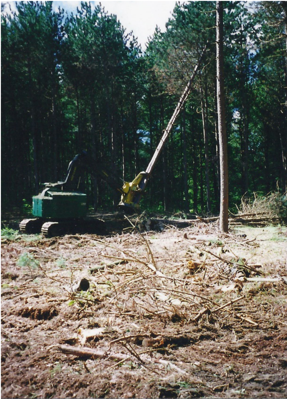
The red pine salvage operation in progress, summer 1999. The vehicle here is called a harvester, whose long boom can reach a range of trees from a single stationary position, thereby minimizing soil compaction and damage to understory vegetation.
